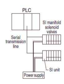
This system can control multiple solenoid valves by using only the communication line from the PLC's communication module (master module) or it can read the signal from the various sensors.
