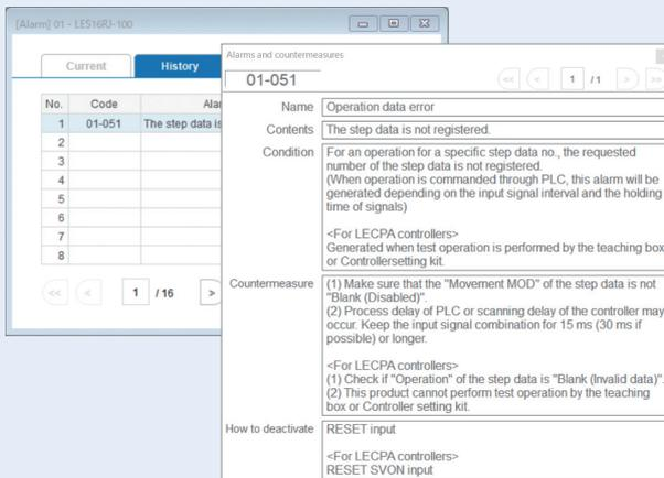
When an alarm is generated, the alarm details and countermeasures can be confirmed.
