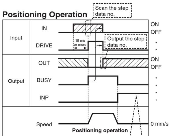
\* "OUT" is output when "DRIVE" is changed from ON to OFF. Refer to the operation manual for details on the controller for the LEM series. (When power supply is applied, "DRIVE" or "RESET" is turned ON or \*ESTOP is turned OFF, all of the "OUT" outputs are OFF.)
