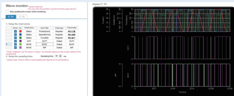
The position, speed, force, and input/output signals' waveform data during operation can be measured.
