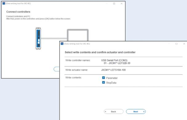
The writing tool can be used to write the connected actuator's parameters and step data to a JXC series blank controller.
