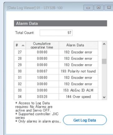
When an alarm is generated, the cumulative startup time of the controller can be confirmed.
