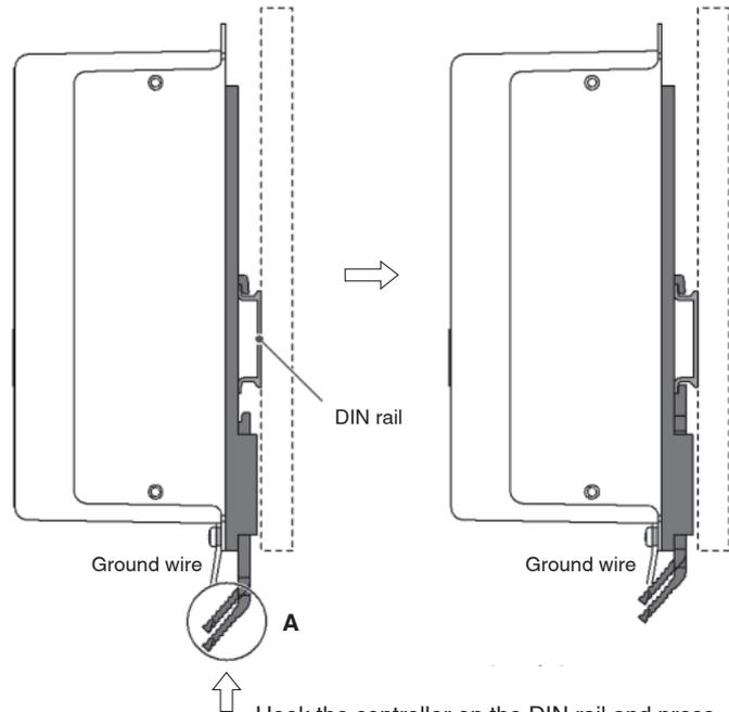
Hook the controller on the DIN rail and press the lever of section A in the arrow direction to lock it.
