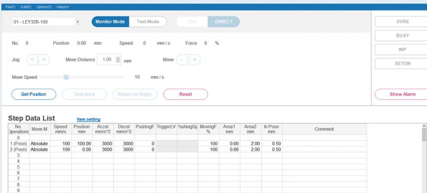
Step data setting, various test operations, and status confirmation can be done on a single screen.
