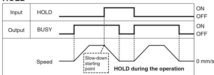
\* When the actuator is within the "In position" range in the pushing operation, it does not stop even if HOLD signal is input.
