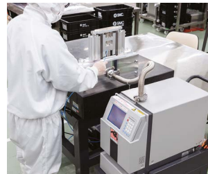
Helium leak testing
