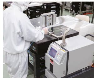
Helium leak testing
